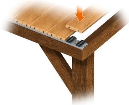
It is the most **universal** version of the product. The Cover Rail is used for all the currently implemented **joists** for the timber deck construction as well for the **deck on posts**. This system corrects rectitude defects, improves the flatness of the structure and protects exterior sides of the wood.
